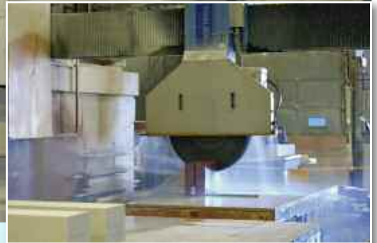
Above: Automated Hensel 567 saw works its way through a 6-foot block.
