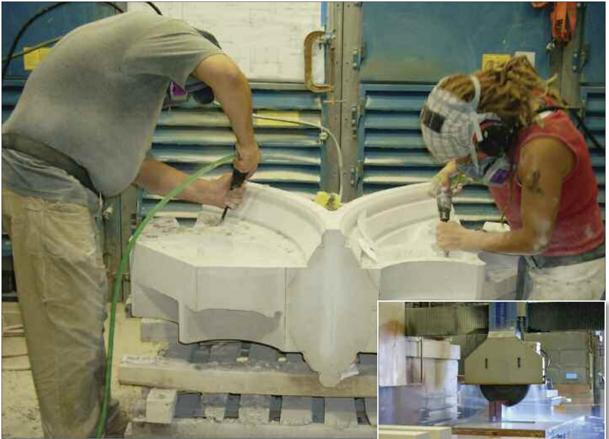
Above: Quarra Stone has over 20 carvers on staff working in two shifts at the plant, which includes work stations designed specifically for carving and handling large pieces of stone. Here, two carvers use pneumatic tools to rough out a limestone tracery piece.
